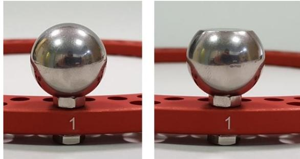
*Reference spheres fixed on an iFIXation® nut: full sphere (left) and truncated sphere (right)*
